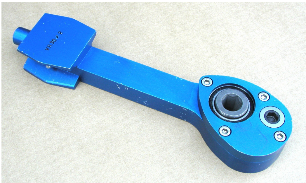
Figure 7.18 : Torque Multiplier (2:1)
