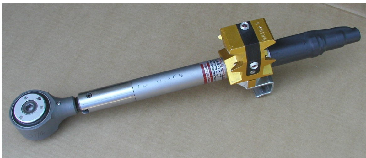
Figure 7.19 : Torque Multiplier (5:1)
