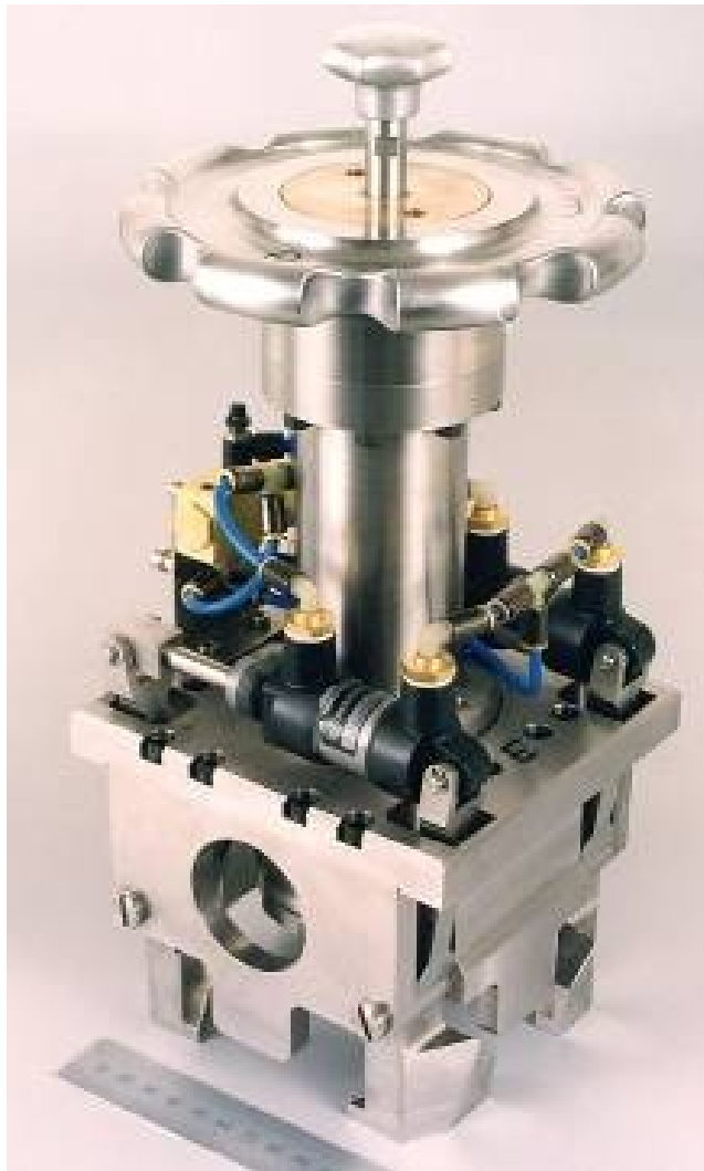
Figure 9.35 : Port Jacking Tool (Typical configured for manual operation)
